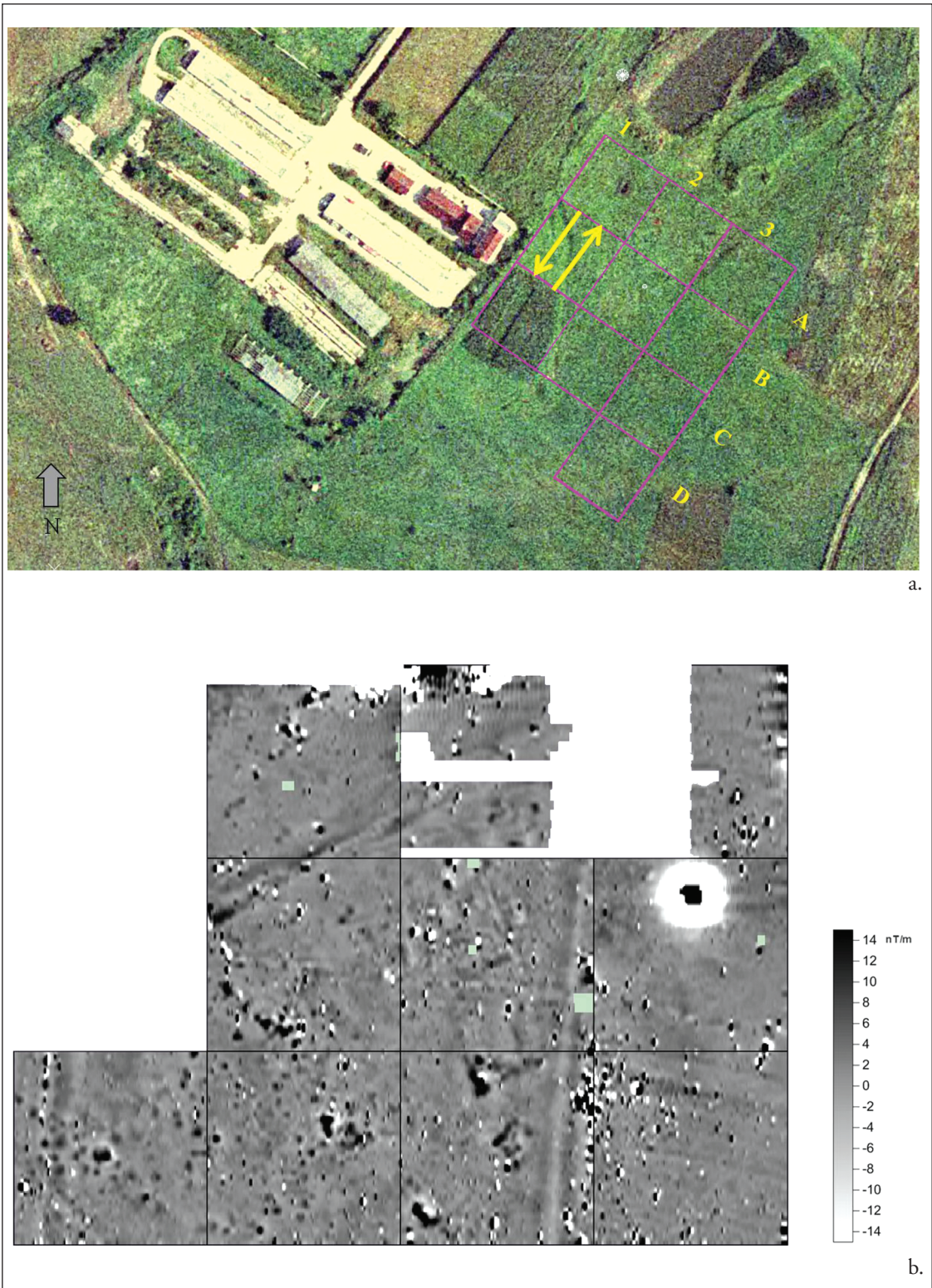
Pl. 2. a. The grid system used for the geophysical survey; b. The magnetic map obtained after processing the aquired dataset.
